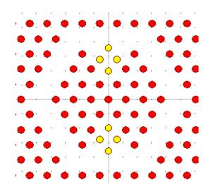
Fig. 2. Schematic structure of PCRR
