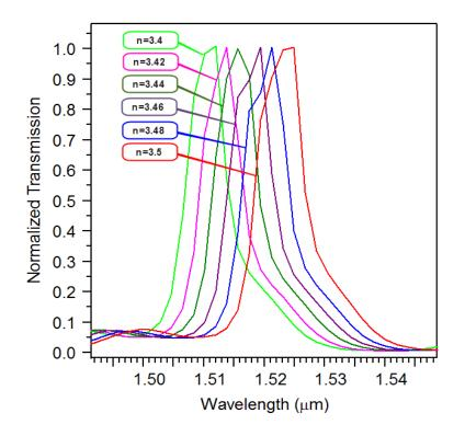
Fig. 6. Normalized power transmission spectra of the proposed CDF for different values of refractive index of of dielectric rods.
