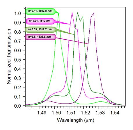
Fig. 7. Normalized power transmission spectra of the proposed CDF for different values of different values of refractive index of inner rods
