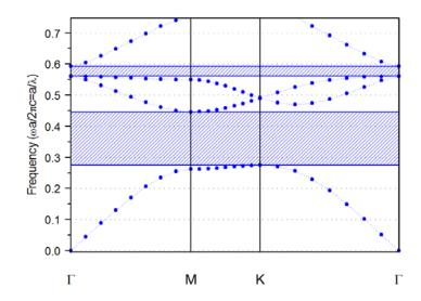
Fig. 1. Band structure of triangular lattice photonic crystal of TM polarized light.
