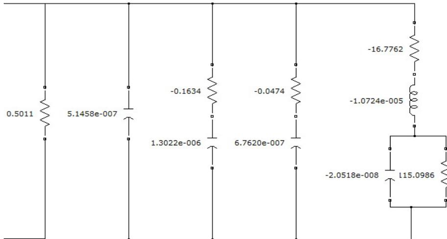
Fig. 8. Equivalent circuit of grid grounding system by VF for conductivity=0.01S/m. Resistors, inductors and capacitances are in,  $\Omega$ ,  $H$  and  $F$  respectively.
