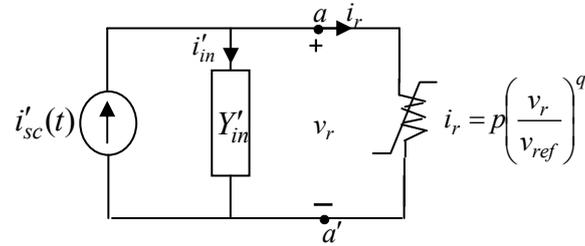
Fig 4. Simplified equivalent circuit of the figure 3.
