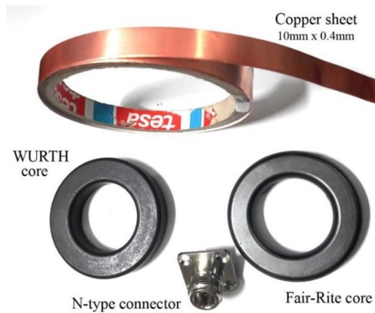
Fig. 3. Materials used in constructing the BCI-probe.
