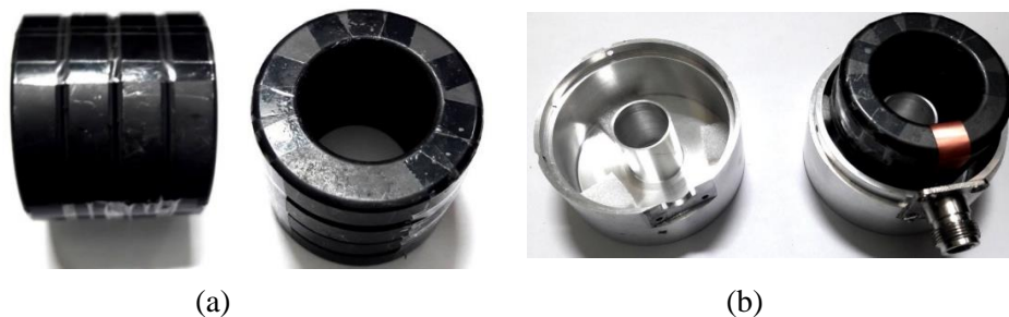
Fig. 4. (a) Assembling four core together (b) The way of fixing the core in the shield.
