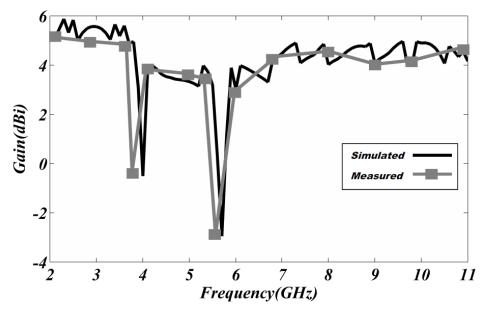
Fig. 5. Mesured and Simulated gain of the proposed antenna
