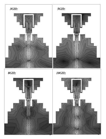
Fig. 6. Simulated current distributions for the proposed antenna at various frequencies
