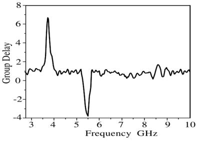
Fig. 8. Group delay of the proposed antenna
