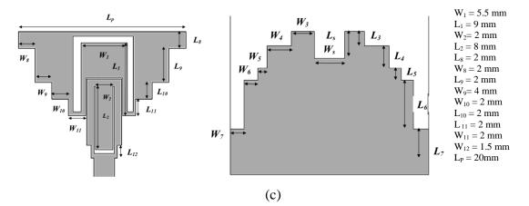
Fig. 1. (a) Design procedure of the antenna (b) Photograph (c) radiation patch and ground plane of the proposed antenna.
