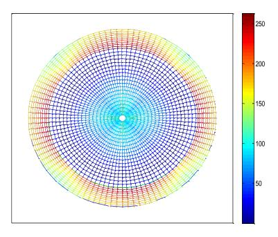
Fig. 2. Field pattern distribution of dual-mode dielectric resonator waveguide filter under HE<sub>11</sub> mode.
