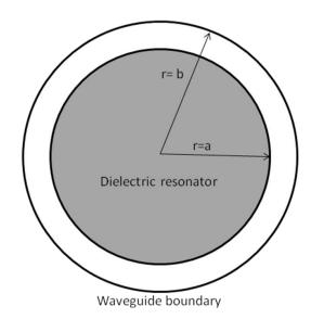
Fig. 1. Cross section of cylindrical dielectric resonator filter
