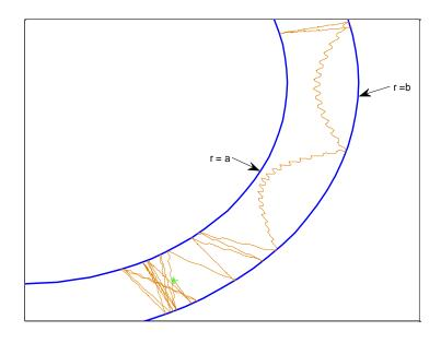
Fig. 3. Electron trajectory for first 30 impacts, Ve=485v, f=2.49GHz
